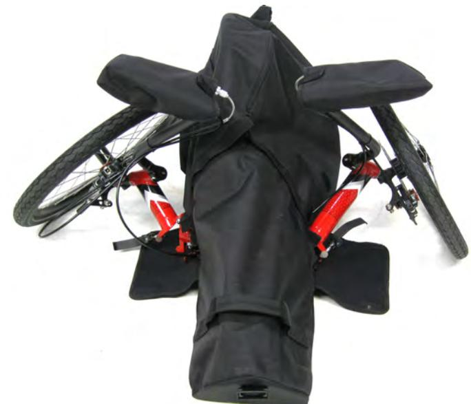
3. Install the elastic wheel covers over the wheels. Ensure the strap slot does not line up with a spoke or valve stem.
