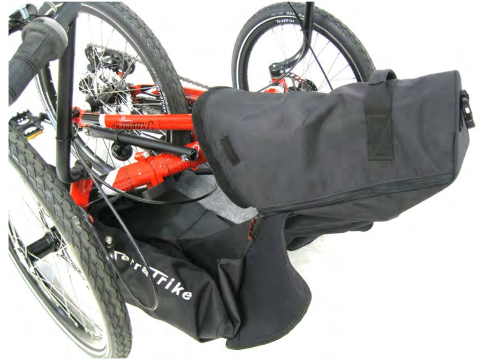
4. Tilt the trike, lifting the chainring guard off the ground. Ensure pedals are positioned as shown for best fit. Note: Pedal position becomes absolutely critical for booms set to "long".
