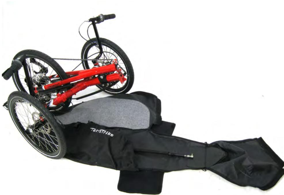
3. Install narrow end of Soft Case around the main tube hinge and zip both sides closed.
