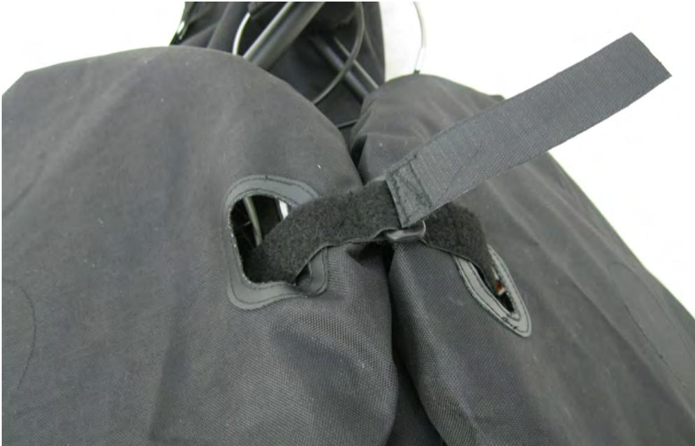
5. Connect the neoprene flaps to the Velcro protecting the outrigger hinges.
