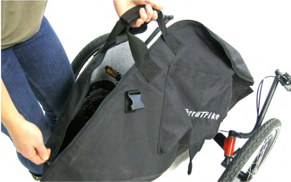
6. Fasten the two halves of the Soft Case together along the Velcro seam. This completes the main tube fold.
