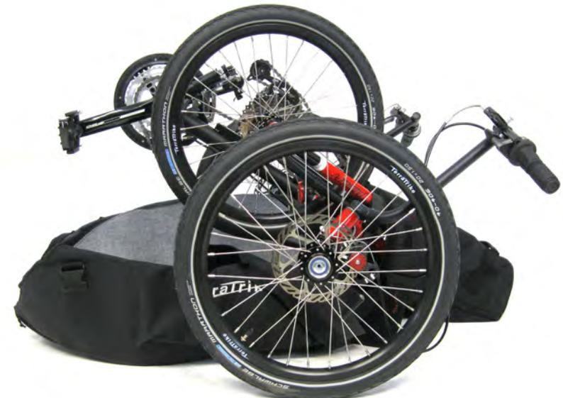
5. Pull up the two large sides of the Soft Case around the crankset and pedals. Zip to close.
