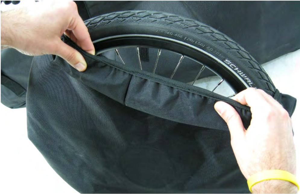
4. Fold the left wheel up first, bringing the wheels together; thread the Velcro wheel strap (supplied with Traveler) through both wheel covers and back onto itself.
