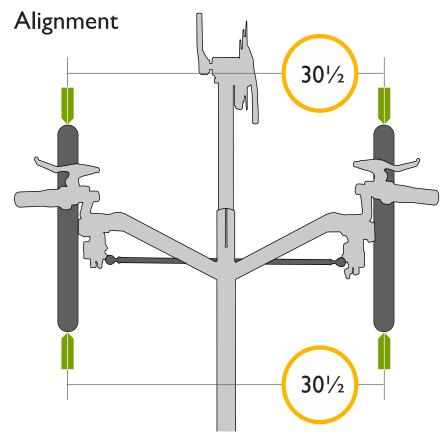
Inflate tires before performing alignment. The All Terrain alignment measurement is approximately 30 ½" (center tread to center tread), though slight variance is possible. Most importantly, make sure the alignment remains neutral with a rider seated in the trike.
